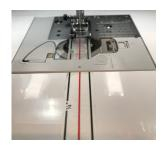
Measures exactly 1/4 inch from center of the red line to center of the black line.
